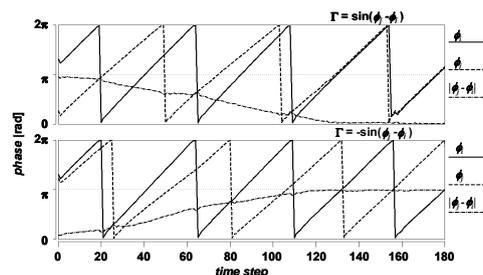
Measurement results of CMOS coupled phase oscillator circuits (synchronized with in-phase and anti-phase)
