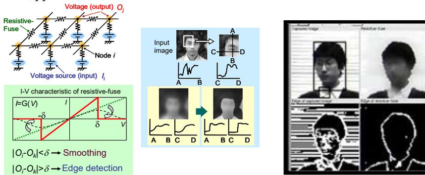
Resistive-fuse network and coarse region segmentation
