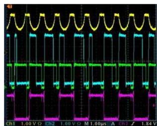
Measurement result of chaos generator circuit (blue waves indicate chaotic PWM signals)
