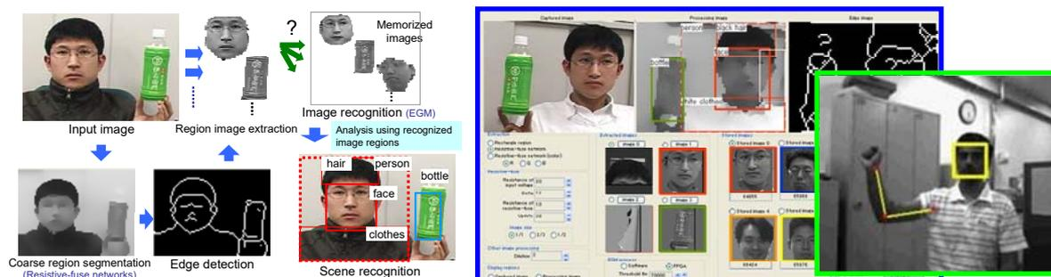
Scene recognition processing flow and outputs of real-time recognition systems.
